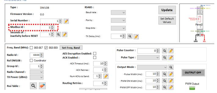
The Modbus ID should be range from 1 to 247, attending to Modbus standard.
